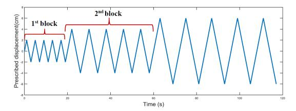
Figure 7. Planned load in quasi-static testing.
