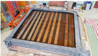
Figure 5. Specimens subjected to imposed current corrosion technique.
