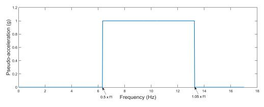
Figure 9. Crenel spectrum used in signal generation.
