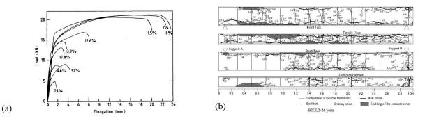
Figure 2. Mechanical effects of corrosion: (a) Ductility loss [17], (b) Concrete spalling [20].
