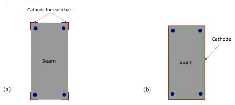
Figure 4. Cathode position (a)  $C_1$  configuration (b)  $C_2$  and  $C_3$  configurations.
