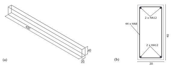
Figure 3. Specimen's design: (a) Geometry, (b) Reinforcement details. - dimensions in centimeters-
